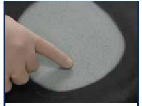
3. Allow to dry 15 minutes and apply a primer surfacer according to paint manufacturer's recommendations.
